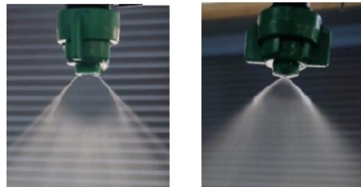
Fig. 4. Spray distribution from flat fan and cone nozzle.
